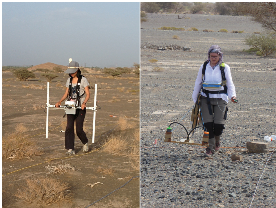
FIGURE 2. The Tübingen survey with the magnetic gradiometer (left) and the LMU team with a total field magnetometer (right).
